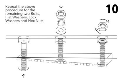
while paying attention to the selected bolts' length(s). Ensure that neither the Bolts nor the Hex Nuts raise above the Counter-Bore hole as they should never touch the rifle's barrel. Tighten, to a minimum of 20 lbs/in of pressure but do not exceed 30 lbs/in of pressure. Confirm the shallow end of the Tilted Rail is pointed towards the butt stock of the rifle and the serrated area of the Rail is pointed away from the barrel.
