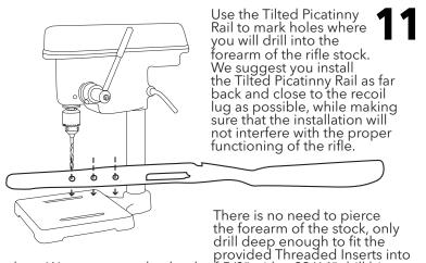
place. We recommend a depth of 5/8" with a 23/64" drill bit. Once the forearm is drilled, screw in Threaded Inserts with a flat head screw driver until they are flush with the forearm. Place the Tilted Picatinny Rail over the Threaded Inserts. First insert the Bolt through Lock Washer, Flat Washer and then through
