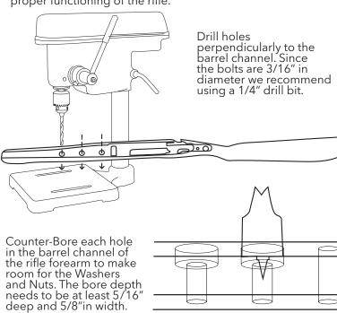
Installing one bolt at a time should make the installation job easier to accomplish.
